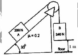
8.a) Determine reaction at supports as shown in figure using the principle of virtual work.
